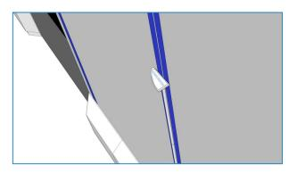
After a maximum of 10 minutes the joint can be tooled. Use the supplied smoothmaker to smoothen out the Hygiseal 3.0 joint and remove excess product. The smoothmaker must be applied under a 45° angle to push the Hygiseal 3.0 into the open joint. Always apply a soapy solution for a good finish and never touch with bare fingers. At a temperature of 23°C the skin formation will follow after ca. 15 min. During this time it is important to keep the fresh joint completely dust-free.
