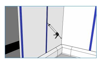
Disperse the Hygiseal 3.0 using a manual or pneumatic 600cc caulking gun under a 45° angle. The consumption of Hygiseal 3.0 is +- 50cc per linear meter. The usage of a pneumatic application tool will provide better results as the same pressure and speed can be maintained. Recommended ambient temperature is between 15°C to 25°C.
