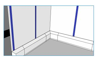
Fix the blue or yellow Hygiseal tape on each side of the joint approximately 2 mm from the edge to create an overlap when applying the Hygiseal 3.0. This overlap will result in a much stronger joint.
