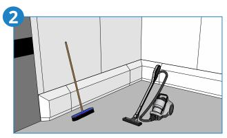
After installation all dust and superficial spots must be removed. Clean the surface and open joint with HygiClean.
