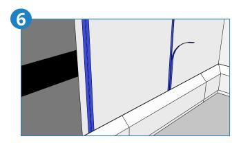
Immediately after smoothening the Hygiseal 3.0 joint, the tape can be removed. Waiting too long can result in the Hygiseal joint being peeled off. Always pull the tape away from the joint. The Hygiseal 3.0 joint will be fully cured after +- 72 hours.
