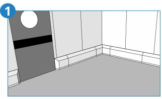
Install the PolySto kerbs and/or B-Hygienic FRP sheets according to the corresponding installation guides. A joint of +- 4 mm needs to be created between each kerb and/or FRP panel.
