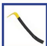
small pinch bar for adjusting the position of the kerbs
