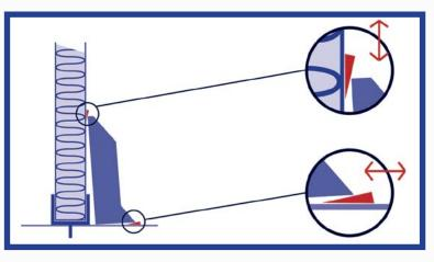
During the course of leveling these sections of kerbs, the best compromise has to be found between following the walls/floor and keeping a straight optical line.
