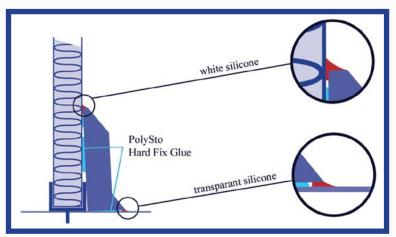
After this period, seal the underside junction to the floor with clear 'PolySto Food Safe Sealant' (silicone), white 'PolySto Food Safe Sealant' (silicone) between kerb and wall and between kerb – kerb.
