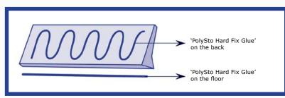
Apply a 'PolySto Hard Fix Glue' line on the floor and to the back of the kerb.
